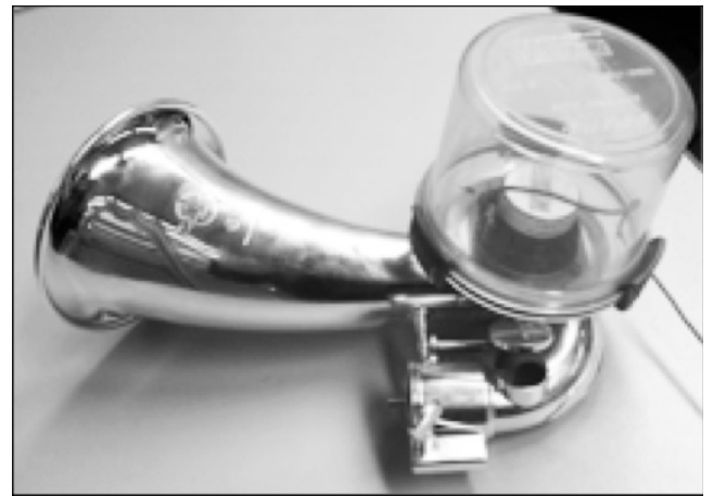
Figure 5. Trombone mouthpiece with an integrated piezo microphone. (Clift et. al 2015)
