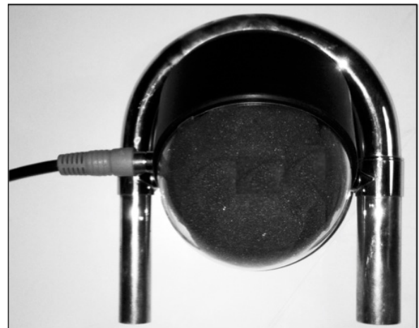
Figure 6. Loudspeaker which has been permanently integrated into a trombone tuning-slide. (Clift et. al 2015)
