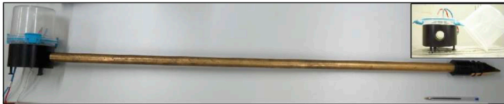
Figure 4. Top: Simplified bass clarinet (a cylindrical tube with a bass clarinet mouthpiece and a reed) with embedded control setup with co-located microphone and speaker. Top right corner: control setup removed from the instrument. (Meurisse et. al 2015a)
