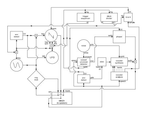
Figure 1. Schematic diagram of the modular system denoting functional blocks and signal flow
